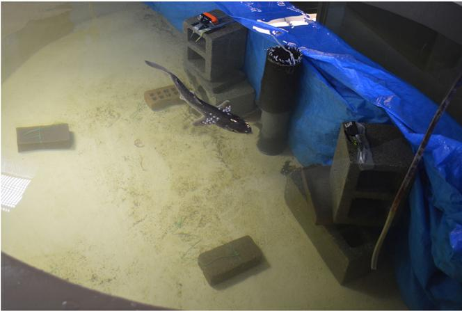
**A Pacific spiny dogfish outfitted with markers along the body and fin swims through a 3D calibrated volume for swimming kinematic analyses.**
